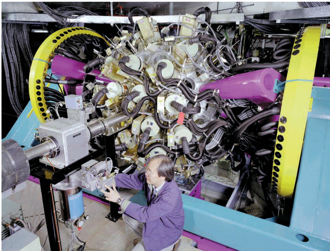
Figure 1. Gammasphere as set up at Berkeley, showing the Compton suppressed Ge detector systems with the beam pipe coming in from the left. Shown in the figure is project manager Dr. I. Y. Lee, who played an important part in the construction and assembly of Gammasphere. Printed with permission of Prof. Mark Riley, author of "Gammasphere—The Beginning... 1993–1997".
